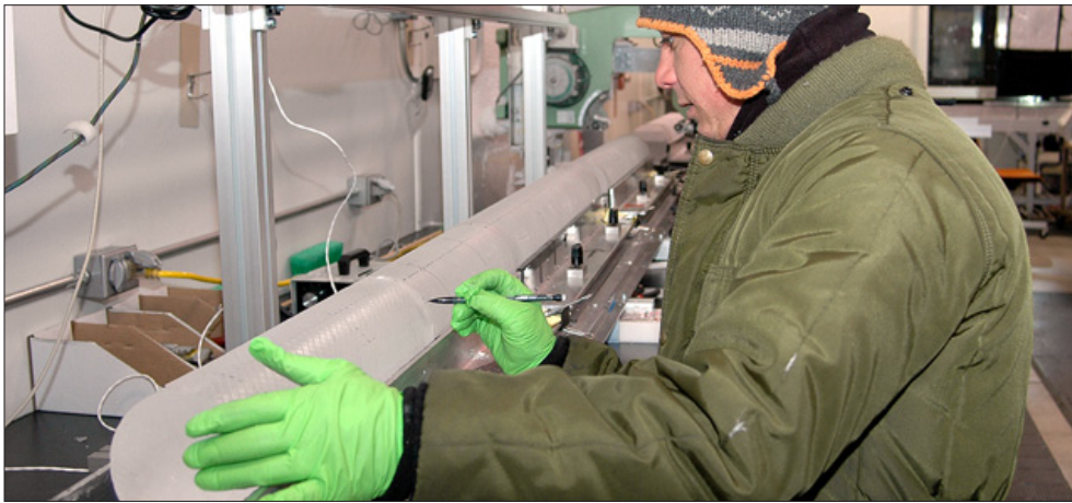
Science technician Tommy Cox measures a section of the WAIS Divide ice core as it begins its journey down the core processing line at the National Ice Core Laboratory near Denver. The technicians will cut the ice so it can be sent to labs around the country for analysis. Photo Credit: Peter Rejcek
