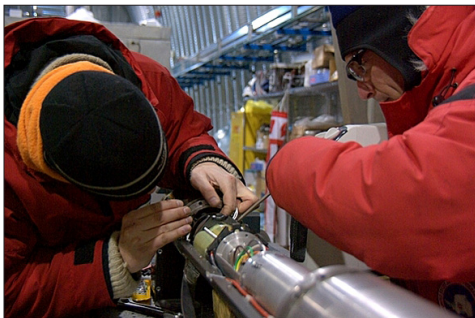
Nicolai Mortensen and Patrick Cassidy work on the sonde electronics of the DISC Drill during the 2009-10 WAIS Divide ice-coring field season in West Antarctica. The drill is the most advanced of its kind on the planet. Photo Credit: Tommy Cox/WAIS Divide
