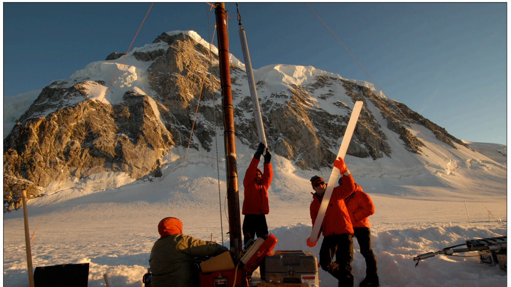
A 2 meter section of ice from Combatant Col is removed from the 3-inch Thermal Drill. Photo: Doug Clark, Western Washington University.
