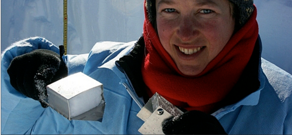
Bess Koffman prepares a snowpit specimen for a density measurement at WAIS Divide during the 2009-10 field season. Photo Credit: Tommy Cox/WAIS Divide
