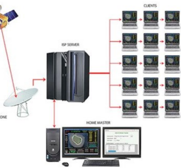
satcom-Receive with server
