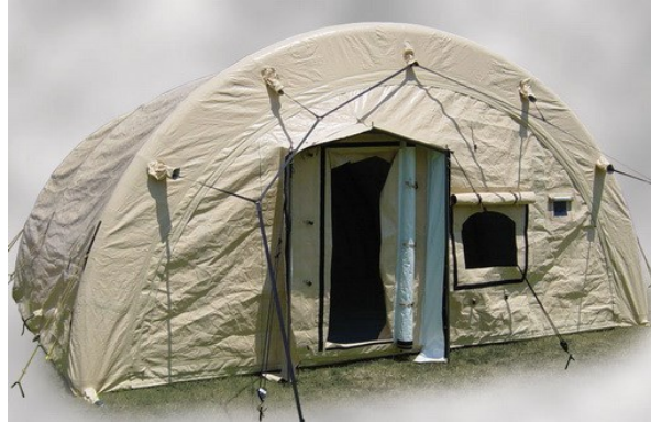
The shelter shown above is the 20 ft. x 21 ft. AirBeam shelter. It can be erected by two men in about 15 minutes using an air compressor. The walls and ceiling are insulated, and there are various feed-thrus for electrical connections and ventilation.
