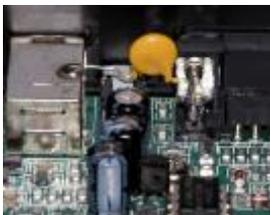
If not already done this modification has to be done before start-up. It has to be done for devices with serial numbers smaller than 765. Just bypass the shield of the USB jack and the metal mounting bracket of the DB37 jack as shown in the picture by a 0.001-0.01 $\mu$ F high voltage capacitor.
